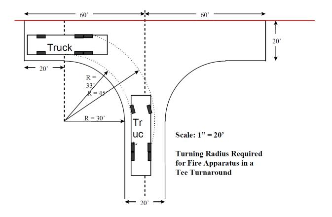
The 20 ft access width is a minimum for use only with an exclusive dire department emergency access way. For roadways or public streets, these access widths must be increased. The end length of 60ft may remain the same, however. Variations of this hammerhead are shown.
