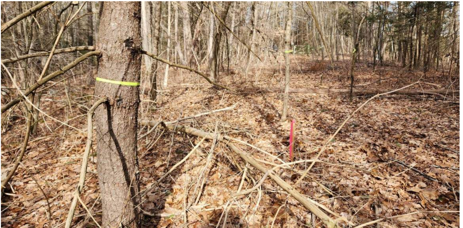
Photo #2: Location of Soil Boring B-2, indicated by wooden stake. B-2 is proposed within the 100-ft and 200-ft Buffer Zones to BVW. Tree removals are required to create a 20-ft wide cleared path centered on the soil borings. Trees proposed for removal are flagged in yellow flagging. Facing northeast.
