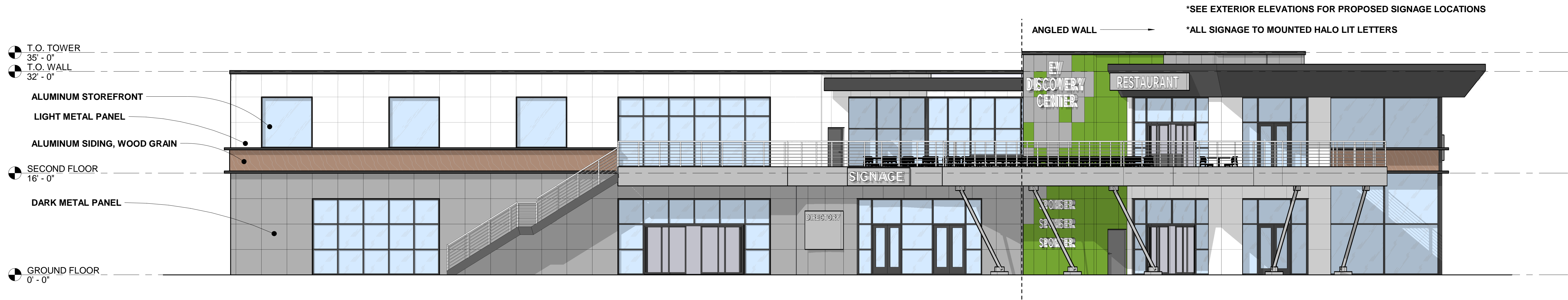
1 EXTERIOR ELEVATION - NORTH (FACING PARKING) (2) SCALE: 1/8" = 1'-0"
