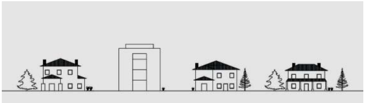
LESS ACCEPTABLE - FLAT ROOF IN PLACE OF PITCHED ROOFS OF OTHER PROPERTIES
