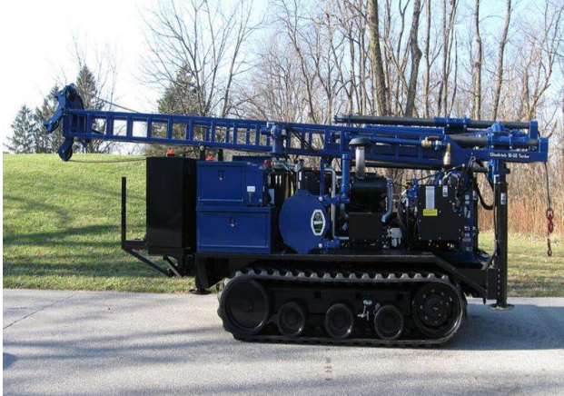
Figure 1: Diedrich D-50 Track Mounted ATV, Geotechnical Boring Rig; Machine Proposed to be Used to Collect Data.
