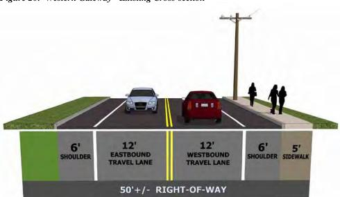
Figure 20: Western Gateway - Existing Cross-section
