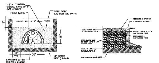
PERVIOUS PAVER DETAIL SCALE: N.T.S.
