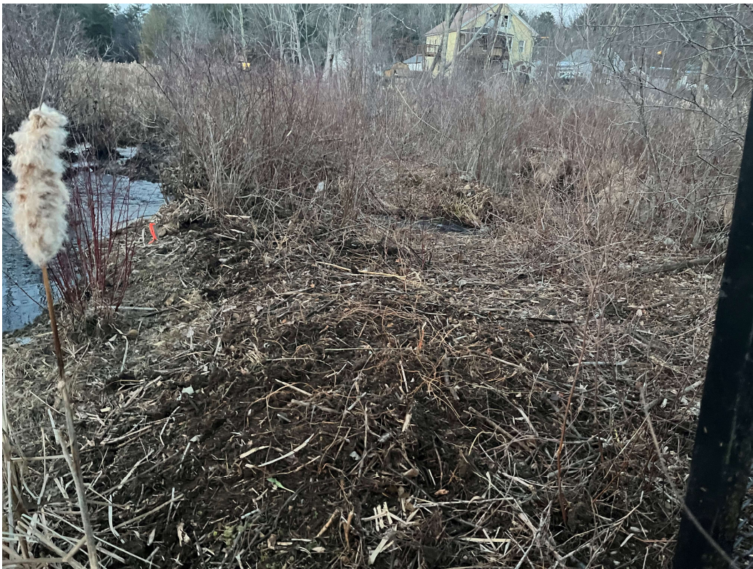
Photo 2 taken by EBT, Inc. on 12/19/2022 – The top of the oak stake which the orange flag to the left of the photo is tied is elevation 580.36. The invert elevation of the outflow pipe shown on Andrews Surveying and Engineering's revised 2005 plan was elevation 577.36. The top of the stake is approximately 1 foot above the
