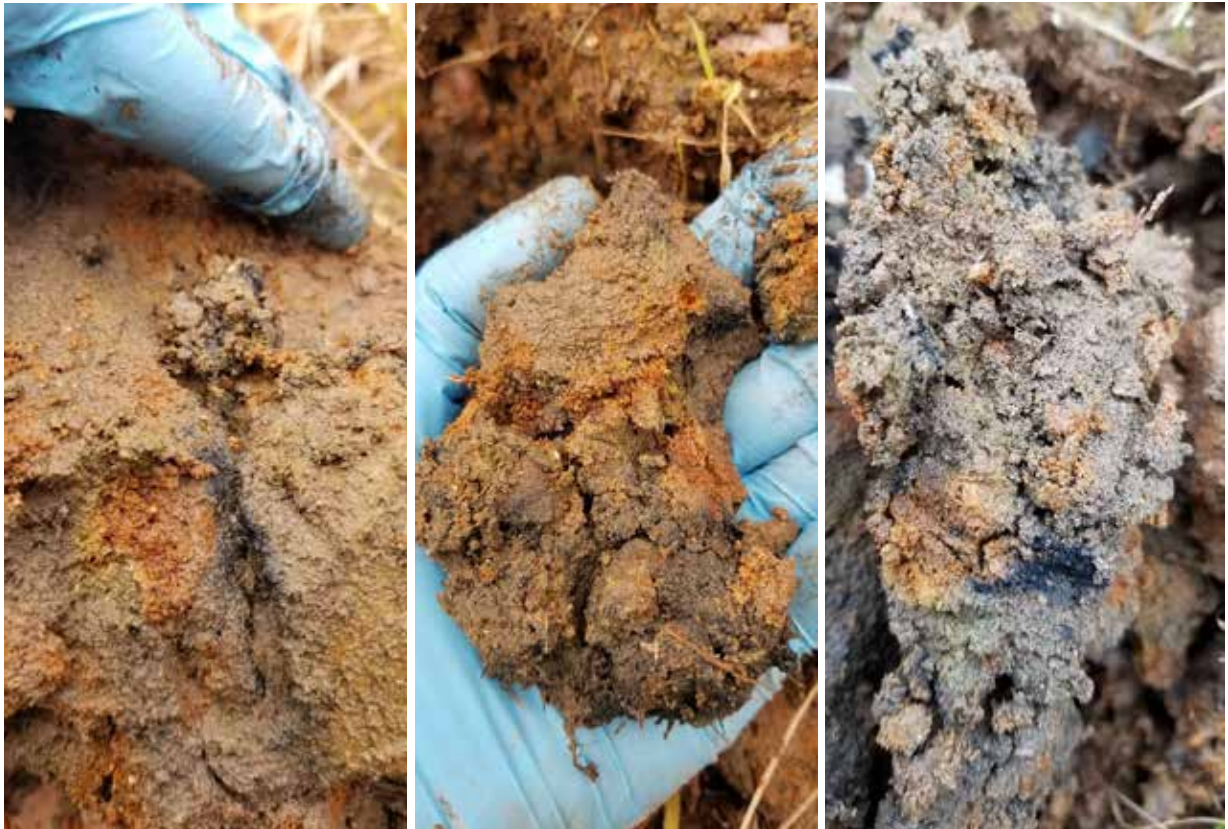
Photograph 12: Wetland restoration soil sample taken at toe-of-slope displaying evidence of strong hydric indicators (e.g., redoximorphic features).
