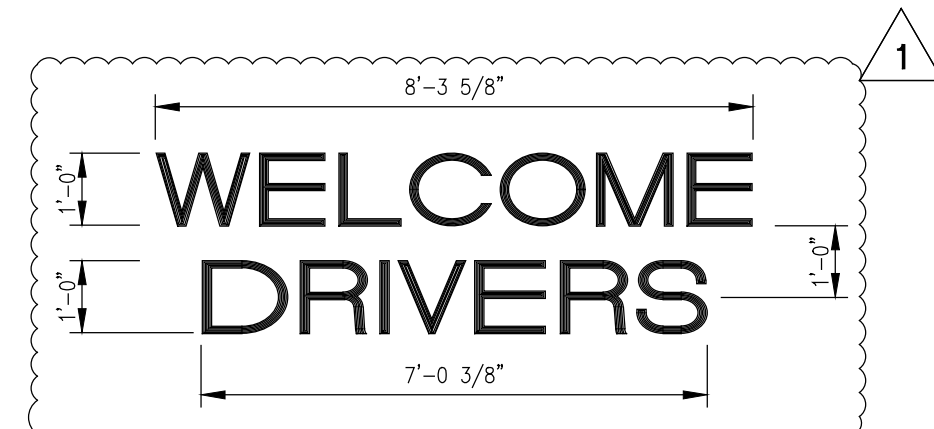
SQUARE FOOTAGE: 16.00 SF. (08) INDIVIDUAL WHITE LETTERS, INTERNALLY ILLUMINATED, DARK BRONZE ANODIZED CABINET
