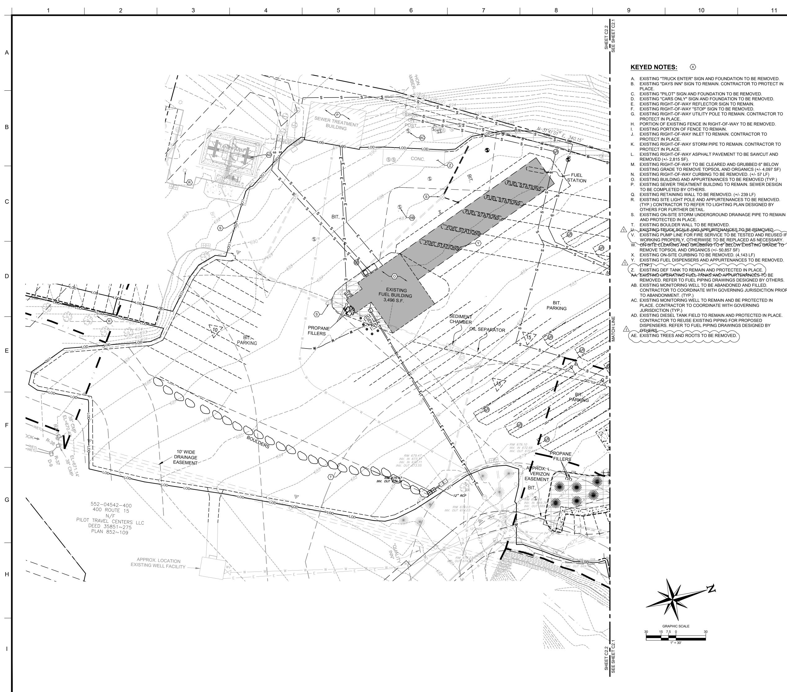
Plot Date/Time: Jun. 24, 20 - 17:48:27 Drawing: P:\Pilot Oil\Sturbridge, MA (400 Haynes Street)-PlL.28950\CIVIL\Drawings\Presentation\PlL.28950 - P - SITE.dwg ;C2.2 - Demolition Plan
