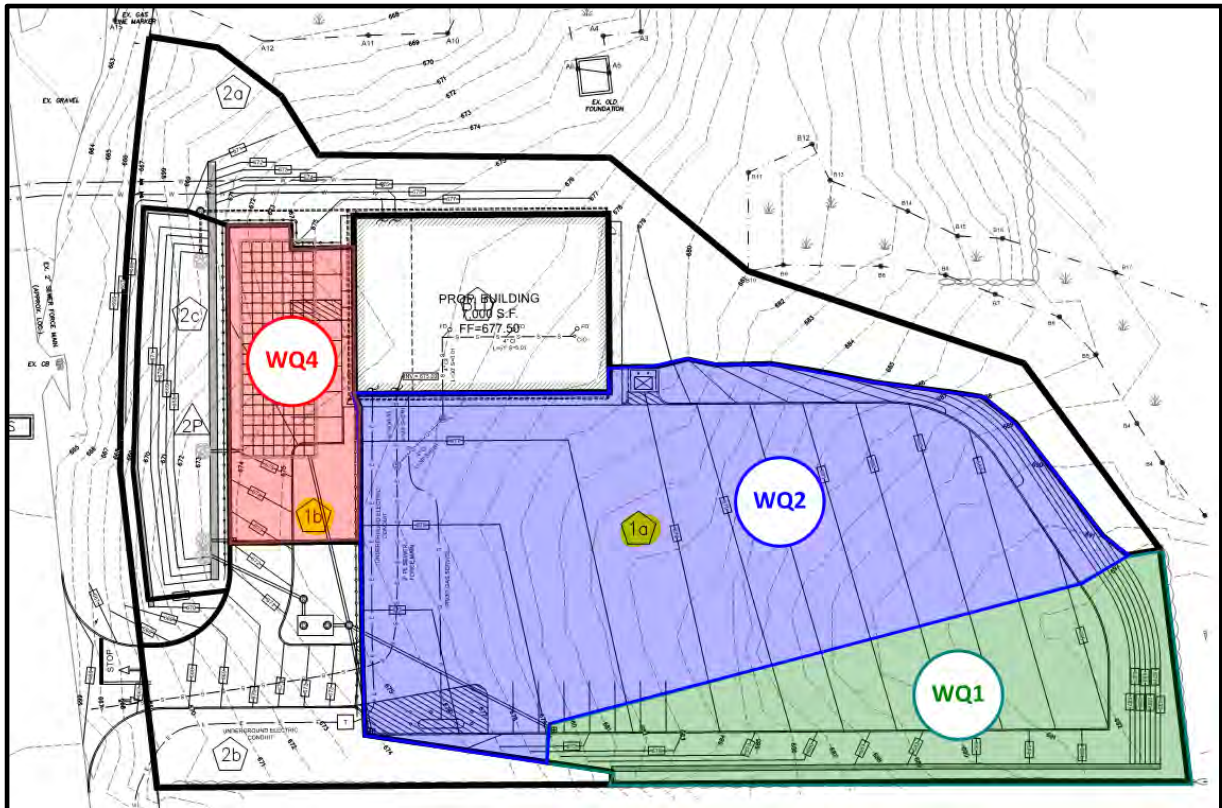
Figure 4. Interstate Towing HydroDynamic Separator Drainage Areas
