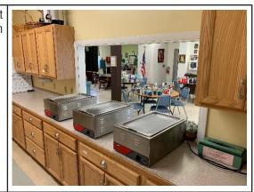
Kitchen food prep area. An exhaust fan was not observed, as the range hood appears to recirculate. The closet door (seen in photo on left side) houses paper goods with the hot water heater. Kitchen sink is insufficiently sized for its purpose.
