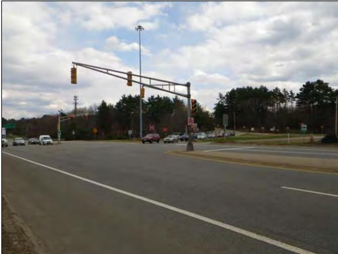
No pedestrian crosswalks or controls are provided at the intersection. Sidewalks are located along the southwestern corner of the intersections. The wide intersection design, coupled with the large radius of the Route 131 channelized lanes, create an auto-centric, unfriendly pedestrian environment at this intersection.
