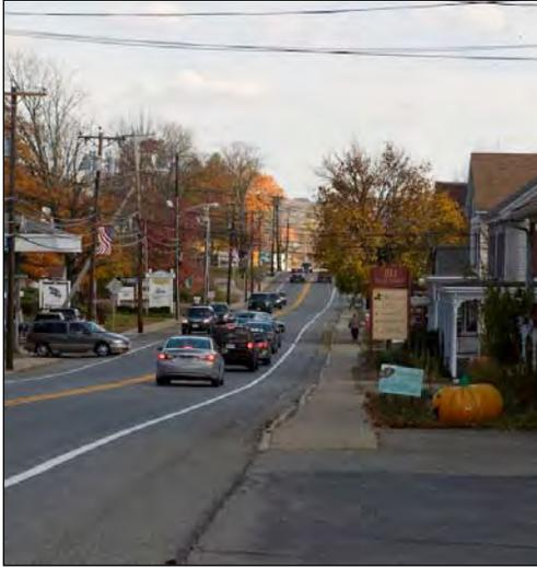
Throughout the Western Gateway, Main Street (Route 20) is a two-lane roadway (one lane in each direction). Shoulders, approximately 6-feet wide, are located along each side of the roadway. Sidewalks are located along the north side of Main Street (Route 20) throughout the entire Western Gateway. On the south side of Main Street, sidewalks are located on approximately one third of the segment. The typical existing cross-section of the Western Gateway is shown in Figure 3 below.
